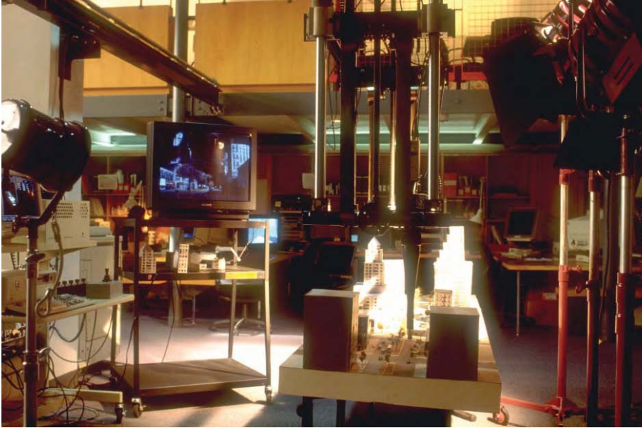
Figure 1.16 – Visualizing zoning alternatives for Broadway on Manhattan’s Upper West Side: Prior to the development of real-time photorealistic 3D digital models, a gantry-mounted miniature camera controlled by computer moves through and records a video on a path in a physical scale model. Photographs of existing and proposed buildings are corrected for parallax and mounted on the physical massing models to create a photo-real effect. (Environmental Simulation Center, 1993)
