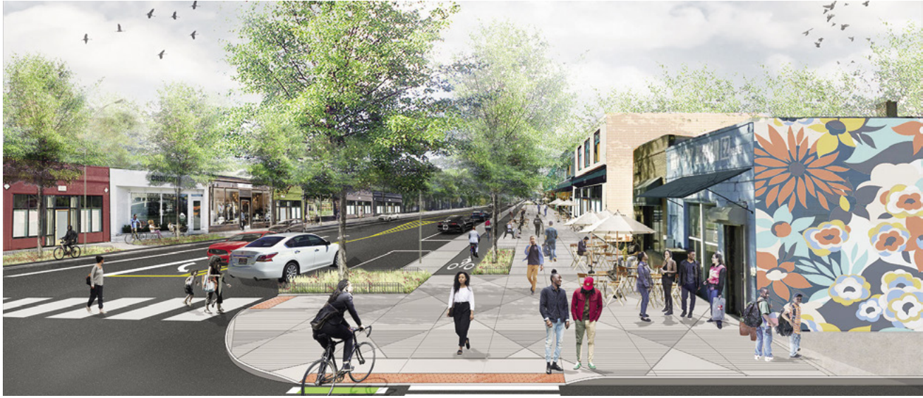
The City of Detroit has undertaken a streetscape project on Livernois Avenue that will add several elements illustrated here, including a bike lane, improved lighting, and extended sidewalks. Credit: City of Detroit Department of Public Works.
