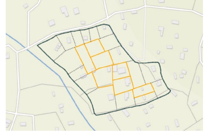
In this Open Reblock map of an informal neighborhood on the outskirts of Harare, Zimbabwe, the dotted lines illustrate how new street segments would connect the seven interior parcels outlined in orange with the existing street network in black. Leaflet | Map data © OpenStreetMap contributors, CC-BY-SA, Imagery © Mapbox
